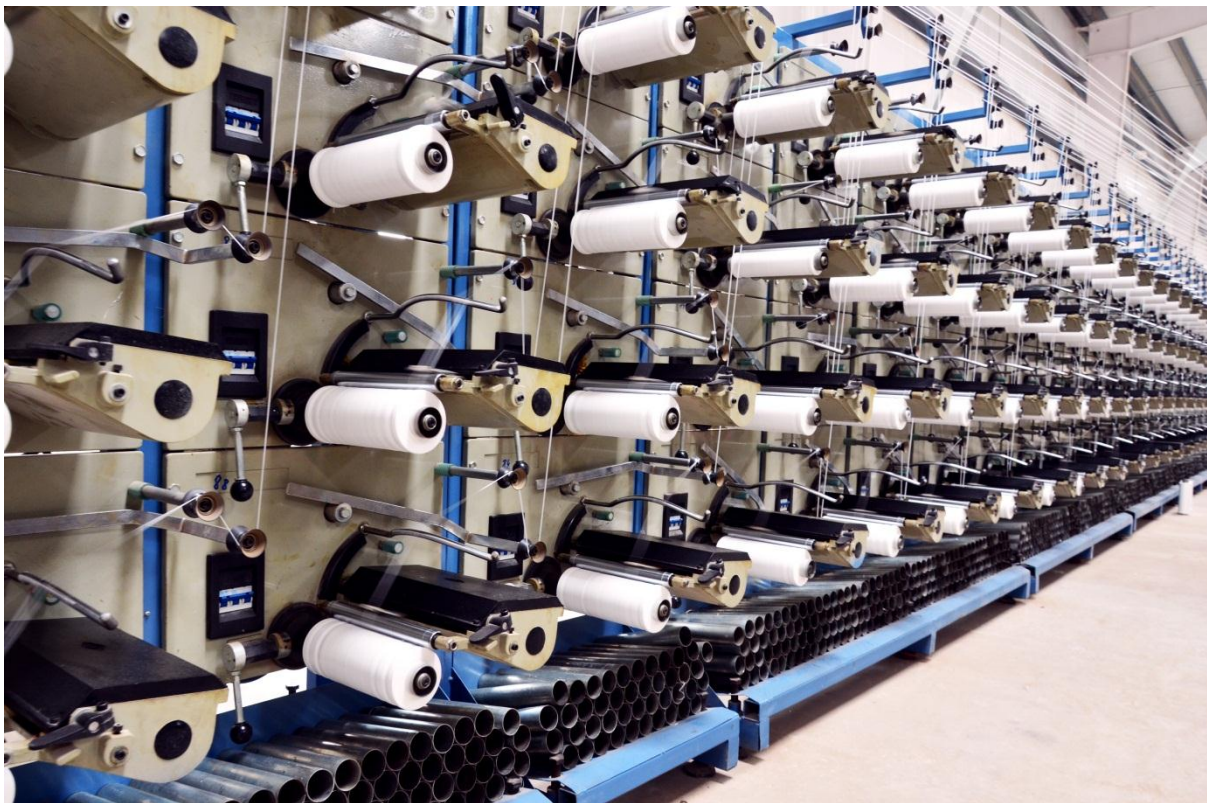
Photograph shows less than half of the 200 electromagnetically actuated automatic precision cheese winders
