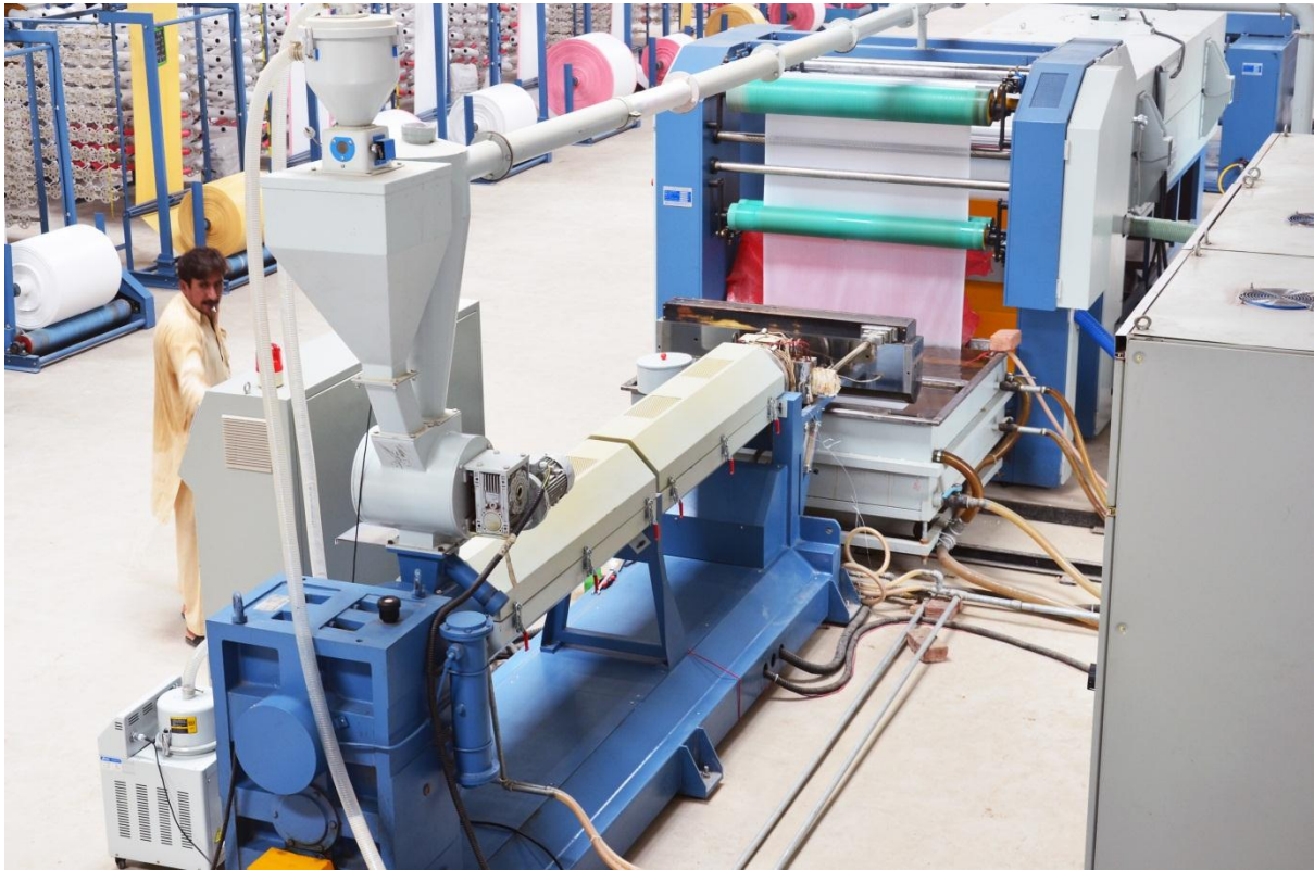
Photograph shows the polypropylene sheet being produced by the extruder
