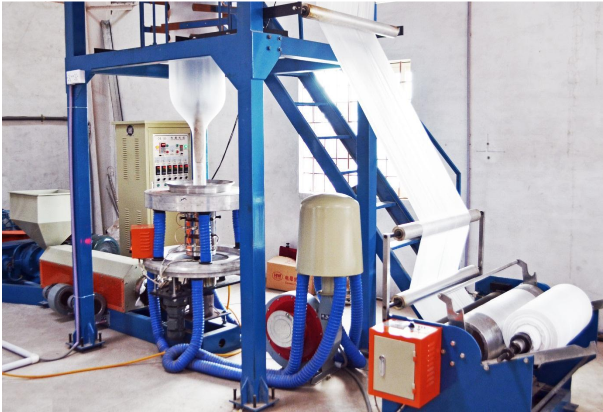
Photograph shows the extrusion and winding sections of the Film Blowing line
