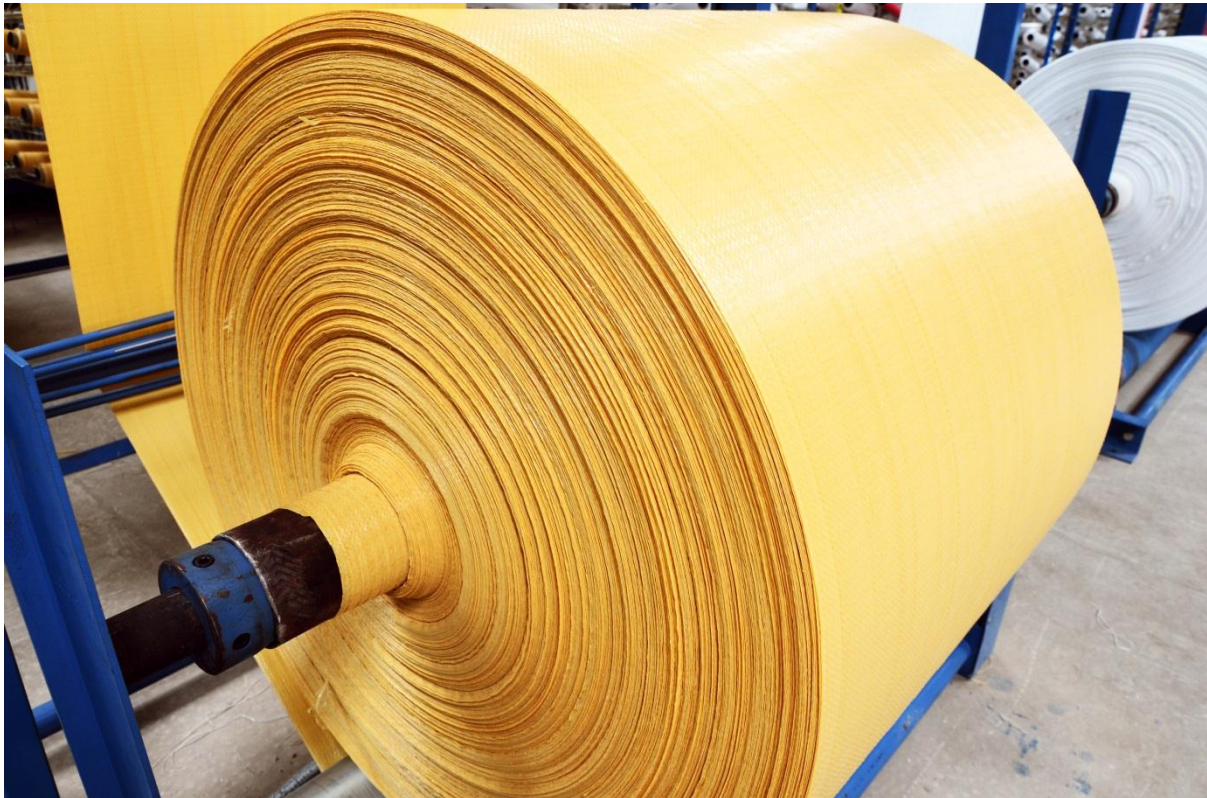
Photograph shows circular woven polypropylene fabric being produced at one of the high speed looms
