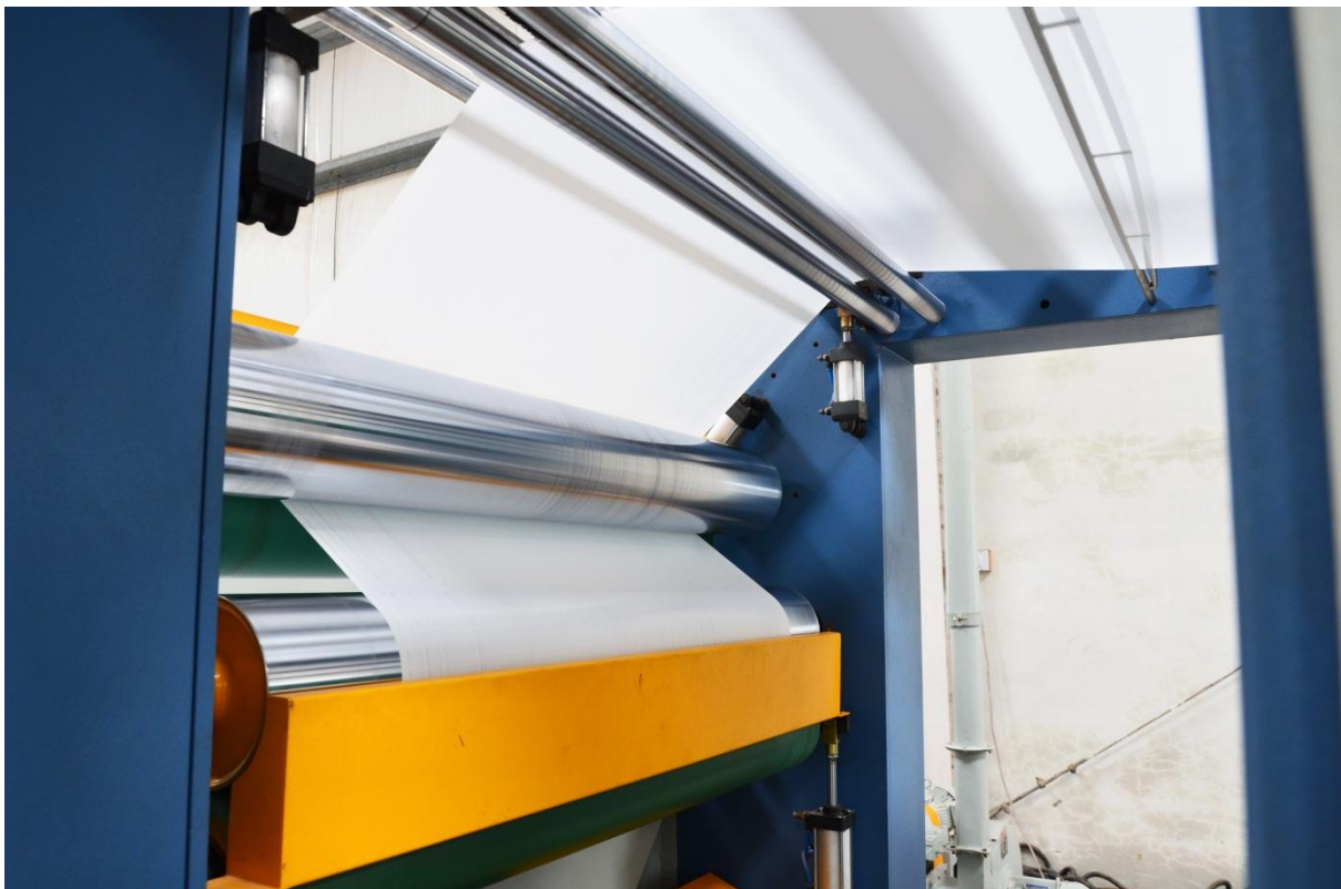
Photograph shows the polypropylene sheet being cut by the extruder's cutting assembly
