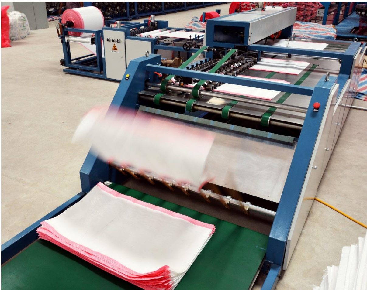
Photograph shows saJWare's Automatic Cutting & Sewing machine preparing feed bags for a client
