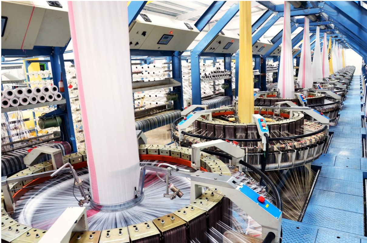
Photograph shows all the 14 High Speed six shuttle looms in operation
