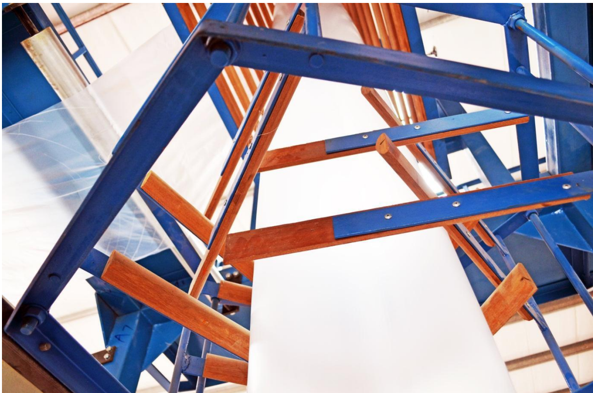
Photograph shows the freshly blown film being transported to the take-ups via the cooling chamber
