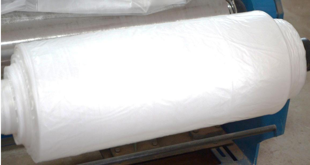
Photograph shows the first test roll of tubular polyethylene film being produced at saJWare Synthetix
