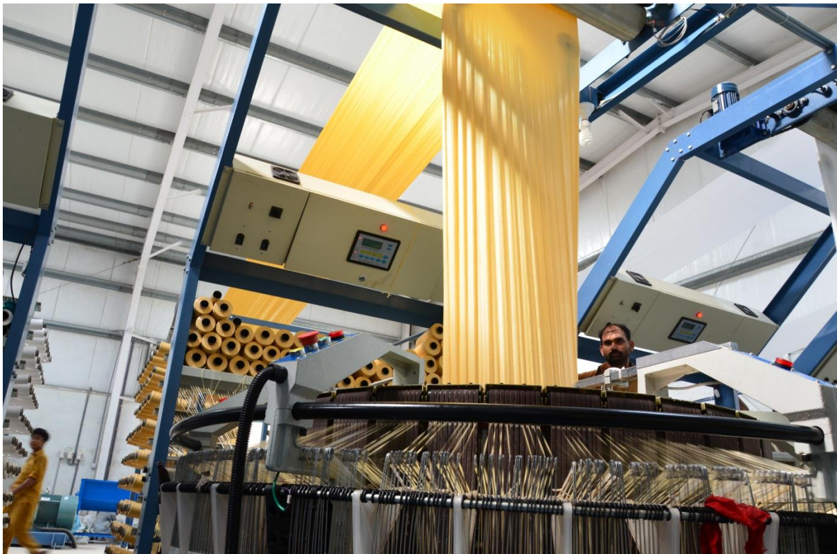
Photograph shows a high speed loom producing beige colored circular fabric for a client
